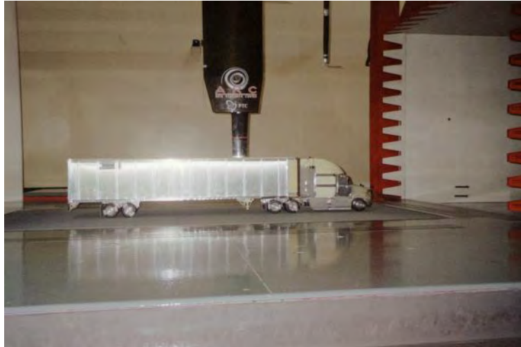
Figure 3-10 1/8th Scale Tractor-Trailer Model in ARC Reduced Scale Wind Tunnel.
