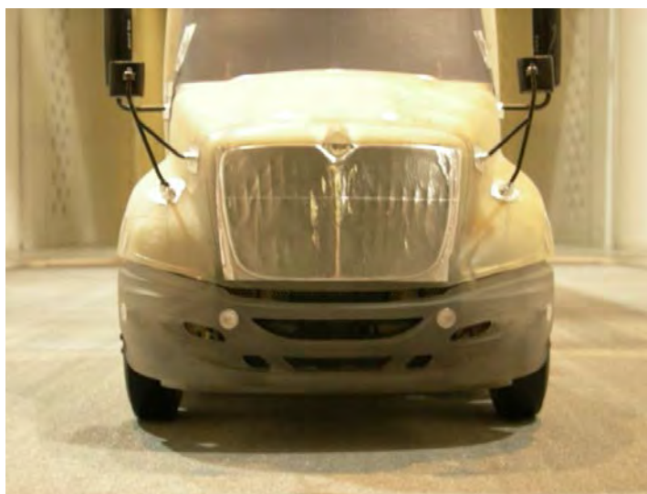
Figure 2-8 Photo of 1/8th Scale Model of a Tractor with the Front, External Grille Covered With Aluminum Tape to Simulate A Closed Grille Configuration
