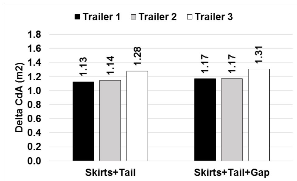
Figure 2-67 Wind Tunnel Performance of Combinations of Bolt-On Trailer Devices; Tractor #4 (ARC Wind Tunnel Data) Pulling Each Trailer
