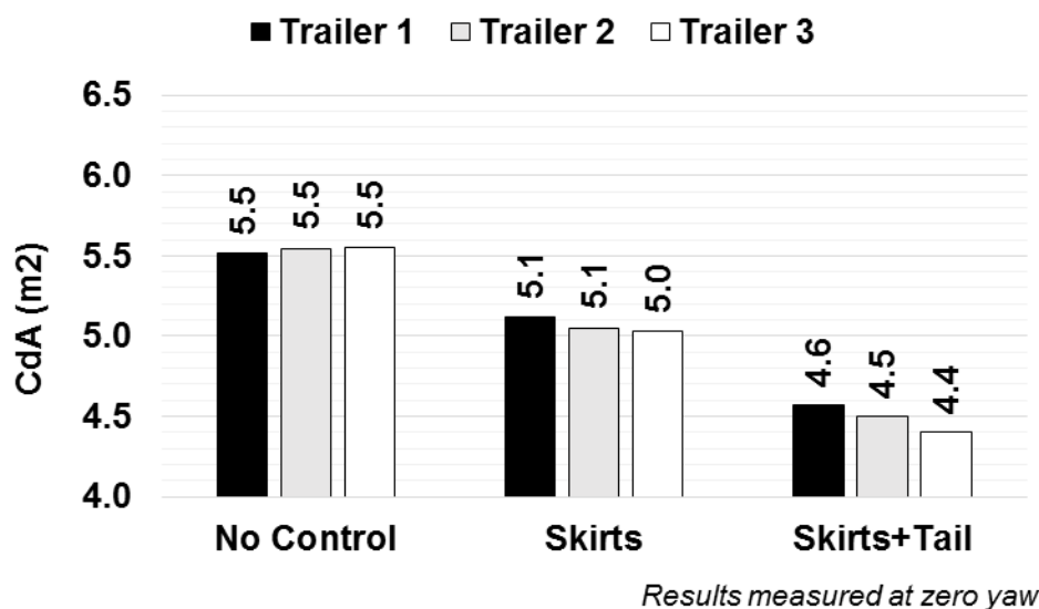
Figure 2-58 Variation in Performance of Trailer Devices due to Trailer Manufacturer; Average Absolute C_dA of Six Tractors Pulling each 53-foot Basic Dry Van Model
