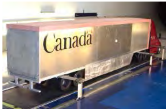
Figure 3-11 1/8th Scale Tractor-Trailer Model in Canada Reduced Scale Wind Tunnel.
